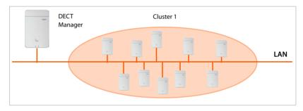
The DECT Manager is connected to the base stations and the PABX via the local network and is therefore not dependent on DECT ranges. Base stations that are far apart can be grouped into different clusters if synchronisation is barely, or not, possible, and is not required. All the base stations of a DECT manager must belong to the same LAN subnet of the DECT manager.
