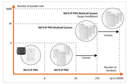
N610 IP PRO Single cell, 8 handsets, 8 simultaneous calls Repeater support for range extension (up to 6) N670 IP PRO Single cell, 20 handsets, 8 simultaneous calls
