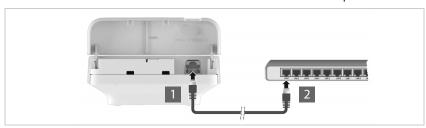
Insert a plug from an Ethernet cable into the LAN connection socket at the bottom of the device 1.
