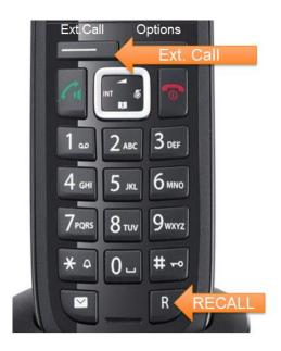
Call Transfer Method: For transferring calls when connected to an advanced PBX trunk (SIP REFER signalling protocol).
