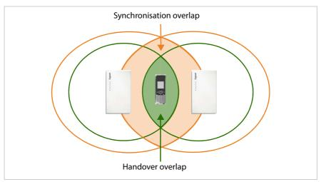
A sufficient number of large overlapping zones between neighbouring cells must be ensured. To achieve synchronisation, the reception must be of sufficient quality to ensure that the base stations can receive one another securely. For a handover, a handset must have a connection of sufficient quality to both base stations. You will find information about possible interferences in the **Defining limit values** section **page 21**.
