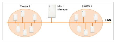
The DECT Manager is connected to the base stations and the PABX via the local network and is therefore not dependent on DECT ranges. This means that you can install separate DECT islands at your location but manage them centrally, i.e., they have access to the centrally configured IP connections, directories, etc.
