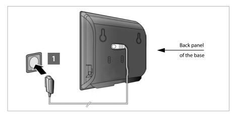
1 Insert the power adapter into the mains socket.
