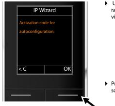
Using the keypad, enter the auto configuration code you received from the provider (max. 32 characters).
