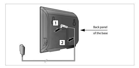
Insert the power cable of the power adapter into the connection socket at the rear of the base.
