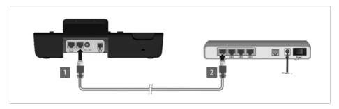
1 Attach one end of the Ethernet cable to the right-hand LAN port on the rear of the phone.
