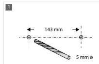
Drill two dowel holes and insert dowels. You can use the wall bracket as a drilling template.
