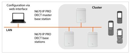
All N670 IP PRO devices build a cluster and synchronise in order to perform handover, roaming and overload balancing for handsets. Synchronisation takes place via DECT or LAN. Up to eight simultaneous calls are possible.
