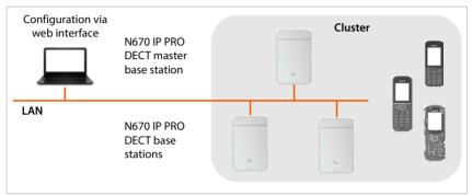
All N670 IP PRO devices build a cluster and synchronise in order to perform handover, roaming and overload balancing for handsets. Synchronisation takes place via DECT or LAN. Up to eight simultaneous calls are possible.
