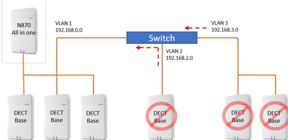
In software 2.33 or higher, it will be possible to install a DECT base station in a different subnet.
