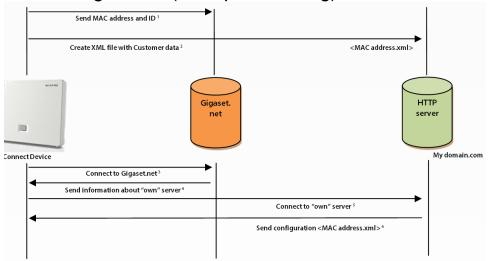
Auto-configuration is the automatic configuration of devices without manual intervention, without any need for software configuration programs or jumpers.
