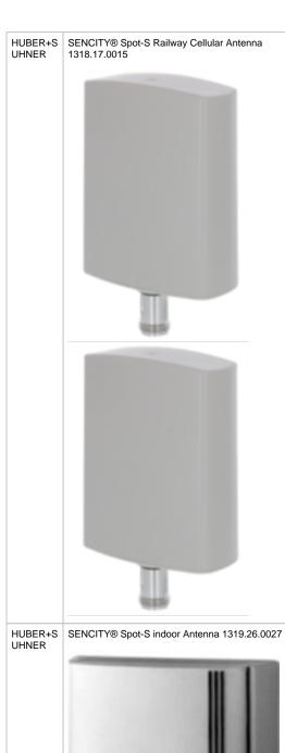
Frequency range (MHz): 1755 -1910 Input impedance (): 50 V.S.W.R: 1.5 3dB beam width (v) (°): 70 Gain (dB): 8 Polarization type: Vertical Max. input power (W): 50 DC grounded: no Connector: Njack female
