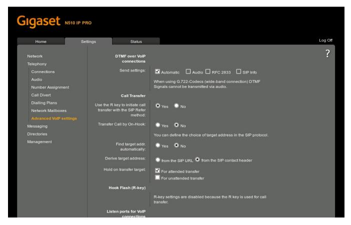
Example N510 IP PRO: Option manually set to "from the SIP contact header".
