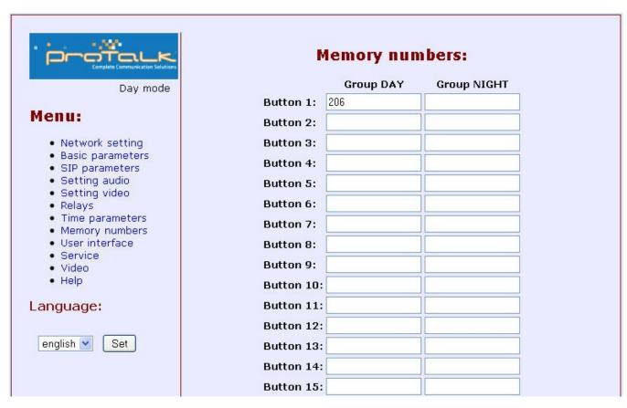
Here you can define which number is dialled when the key is pressed, in this example number: 206.
