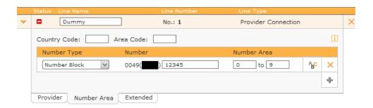
6. Add the external "dummy" number in PBX2 to the user, which one is allowed to call to external destinations. Make sure that the Display Number is set, too.
