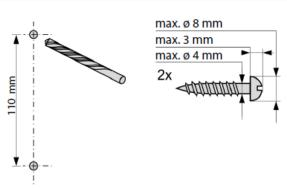
Fix the device to the wall with two screws:
