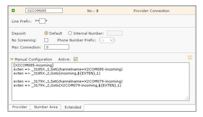
In the manual configuration, we defined that every incoming number that starts with 3179 will be handled by the line with the name X2COM079, the numbers starting with 3185 will be forwarded to the line with the name X2COM085.
