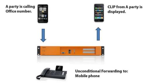
To enable A number forwarding in your Gigaset T300/500 PBX system, you need to activate the No Screening feature in the extended line settings.
