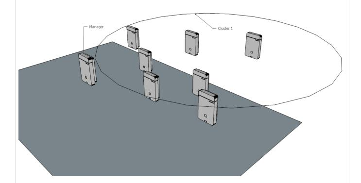
The DECT Manager is connected to the base stations and the platform via the local network and is therefore not dependent on DECT ranges. Base stations that are far apart can be grouped into different clusters if synchronisation is barely or not possible, and is not required. All the base stations of a DECT manager must belong to the same LAN subnet of the DECT manager.
